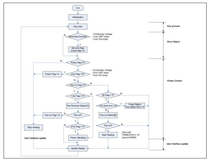
Figure 3-2 Software Diagram
